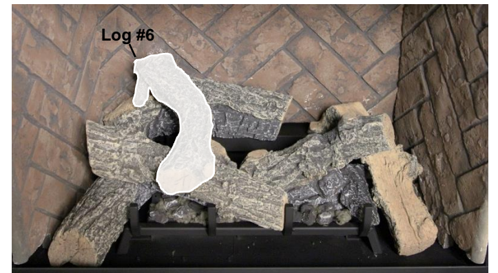
Step 7: Place Log #6 onto Log #1 and Log #5 making sure to position between the end and center flames evenly. There should be no impingement of flames or sooting may occur.
