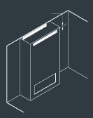
Framing to ceiling with vents at front and back
